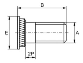
For plate thickness, min = 1.5Head diameter E = 6
